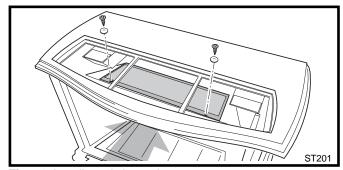
Fig. 21 Install catalytic combustor.
